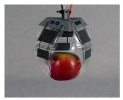
Joints (SES joints) to enable its high performance. The SES joints are very small and light joints, made up of thin plastic films filled with liquid dielectric oil. These bots are specially made for small-scale robotic systems of only a few centimetres in size, where the limited space severely restricts the choice of actuator technologies.
